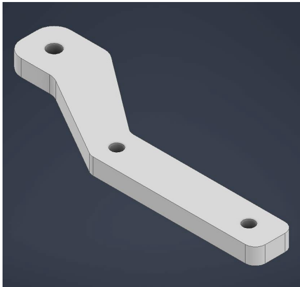
Figure 2.4.13. Right connecting arm
